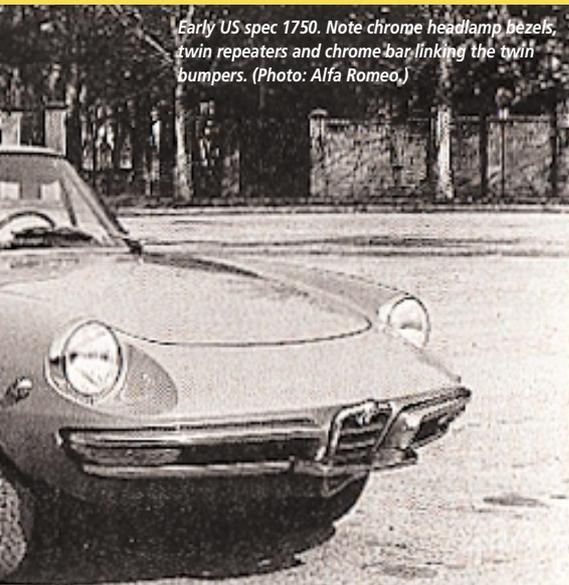
*Early US spec 1750. Note chrome headlamp bezels, twin repeaters and chrome bar linking the twin bumpers. (Photo: Alfa Romeo.)*
